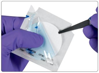
Utilizing sterile forceps, peel back the film and separate the blue paper from the membrane. Remove the membrane with the forceps.
