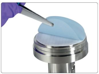
Place the membrane and blue paper on a wet filtration support. When wet, the blue paper curls enabling you to easily remove it using your forceps.
