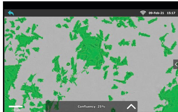
To calculate estimate cell count click [Count](#). The confluency and cell count masks can be adjusted. Click the arrow on the right side of the screen to open the two slide bars.
